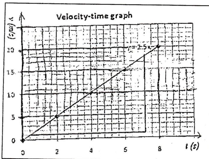
c) Gradient:  $\text{grad} = \frac{\Delta v}{\Delta t} = \frac{18}{7.2} = 2.5$
